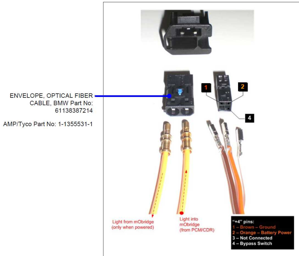
Figure 5 Fully disassembled mObridge wiring assembly
