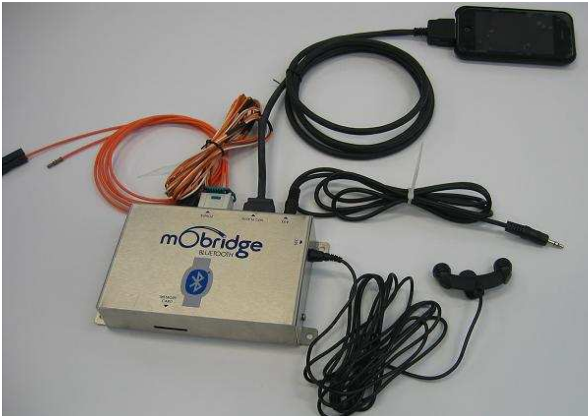
Figure 7 Connections for the mObridge Audio & Bluetooth Interface
